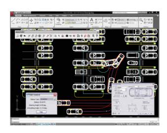
Add a better perspective of visualization to your simulations. Use realistic plan views of vehicles and modify colors, line types, and hatching of vehicle bodies and travel paths.
